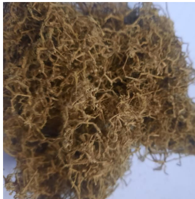
Fig. 3.14 – Fiber Obtained from Pine Extract Production Waste.
