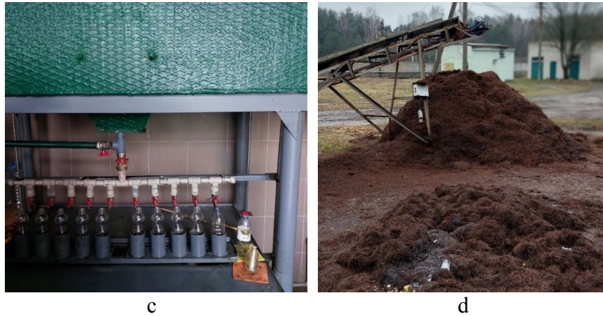
Fig. 1. Production of pine extract and essential oil: a – grinding of pine branches; b – water extraction of active substances in a sealed container; c – distillation of pine extract; d – solid waste from pine extract production.
